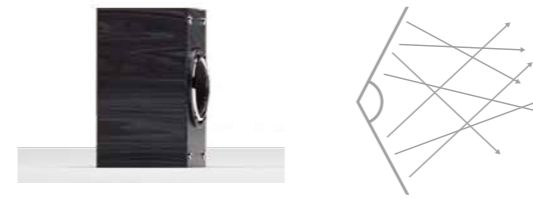
Cone-shaped diaphragm better diffuses sound
